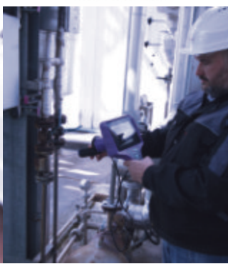
STEAM TRAP INSPECTION
